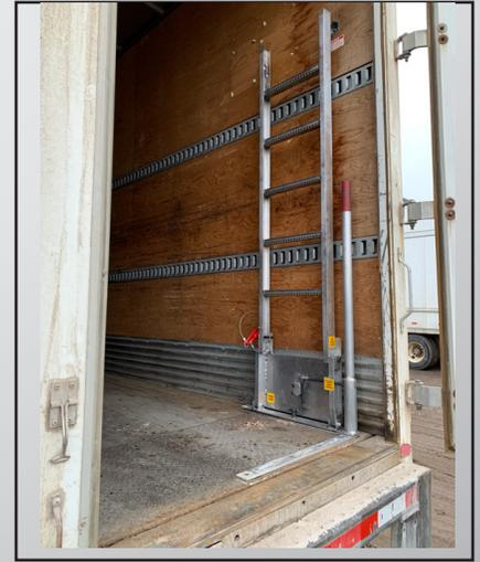
Ladder stored out of the way to allow for forklift access.
